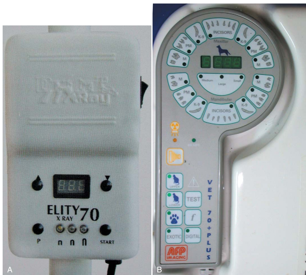
FIGURE 13-2 Control units. A , A simple control allowing the user to set the exposure time and make the radiograph. B , An anatomical interface without timer selector.
