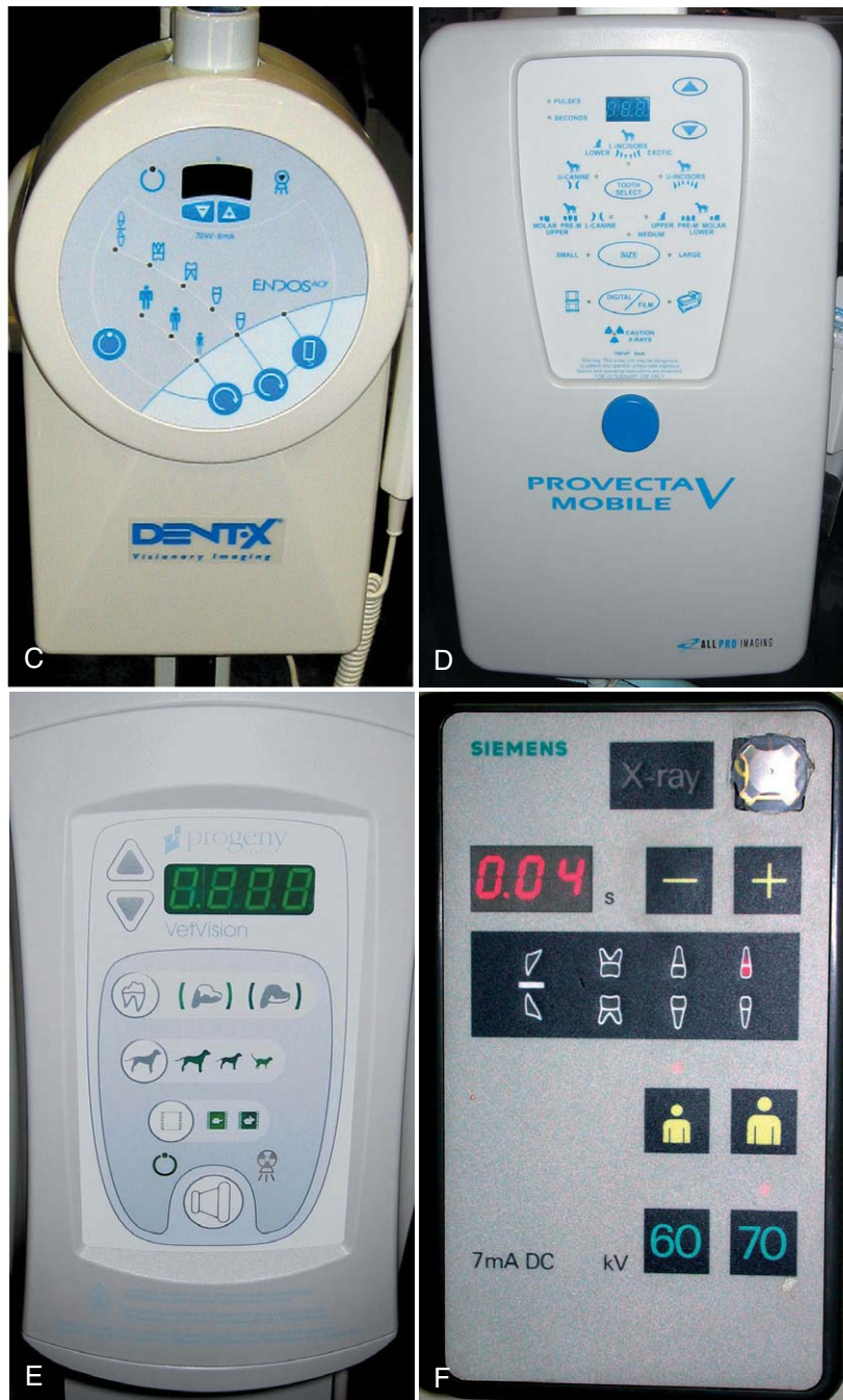
FIGURE 13-2, cont'd C–E, Anatomical interface with timer selector. F, The authors' unit, which has been in service for more than 12 years, has a timer and kV selector. The only buttons used are the exposure time selector and the activation button. The plastic covering has long ago worn off the exposure button.
