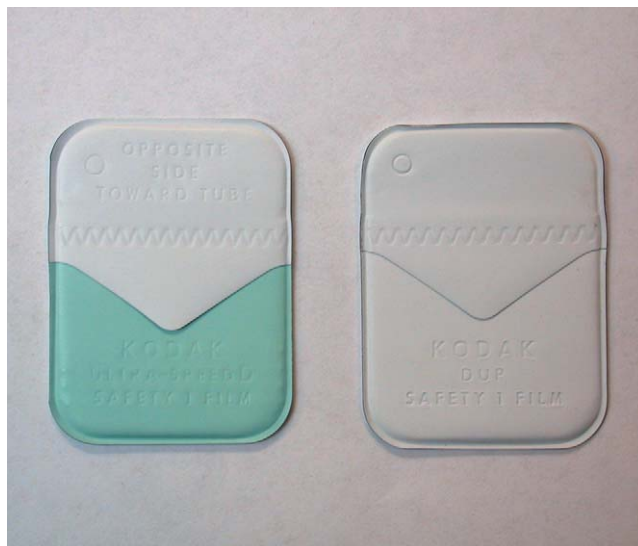
FIGURE 12-3 A film packet with normal x-ray-sensitive film ( left ) and a packet with visible light-sensitive duplicating film ( right ).
