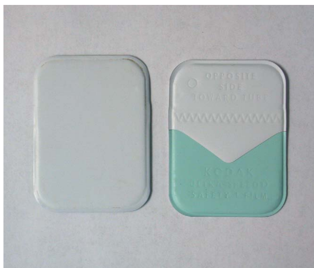
FIGURE 12-4 The front of the film packet ( left ) that is positioned toward the x-ray tube is relatively featureless except for the orientation dot. The back of the film packet ( right ) often has a tab to assist opening the packet and may also have other identifying marks.
