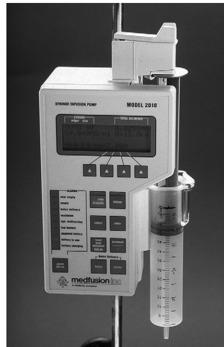
Figure 22-8. Battery-supported syringe infusion pumps simplify the administration of small quantities of drug once the machine is programmed with the animal's weight, the dose ( \mu\text{g/kg/min} ; \mu\text{g/kg/hr} ; ml/hr), and the concentration of the solution ( \mu\text{g/ml} ; mg/ml).
