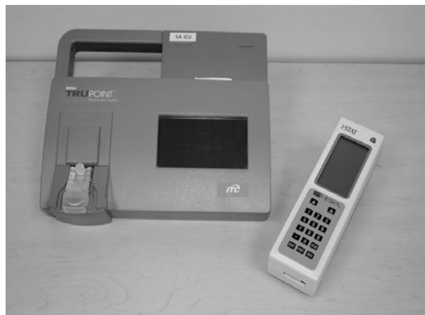
Figure 8-11. Point of care pH and blood gas analyzers (ERMA Trupoint; 1-Stat) facilitate the immediate acid-base analysis of arterial and venous blood samples. Most analyzers also determine electrolyte and lactate values.
