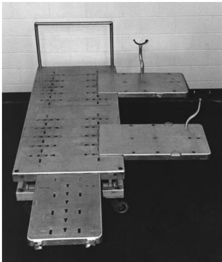
Figure 16-25. Portable hydraulically operated table with removable adjustable head and leg supports. (Kimzey Welding Works, Woodland, CA.)
