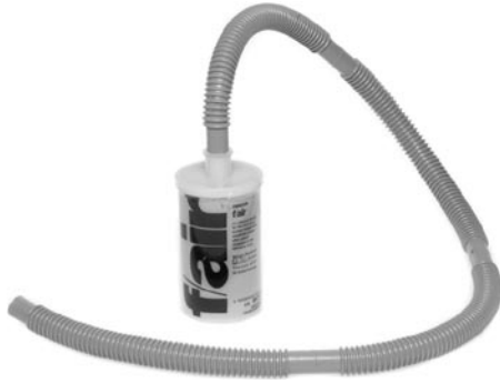
Figure 16-23. Charcoal canister for passive collection of waste gas from the pressure relief valve. The free end of the hose connects to the pressure relief valve.
